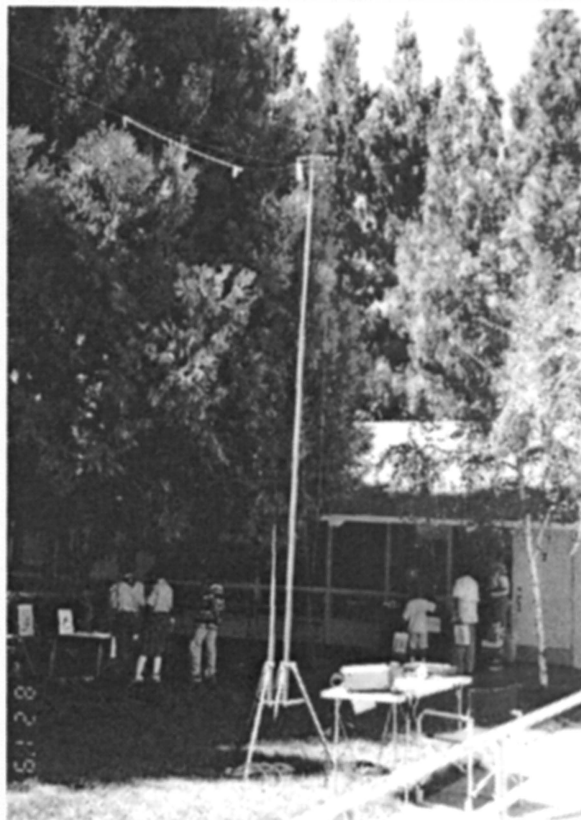
10 and 40 meter dipoles on a 15 foot tripod mast.
